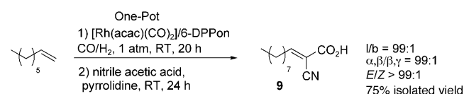
Scheme 8. One-pot RTAP hydroformylation/Knoevenagel reaction towards the \alpha -cyano acrylic acid derivative 9 .
